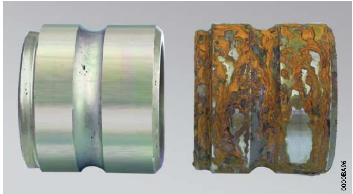
Figure 2 Coated and uncoated part after 24 h in the salt spray test
