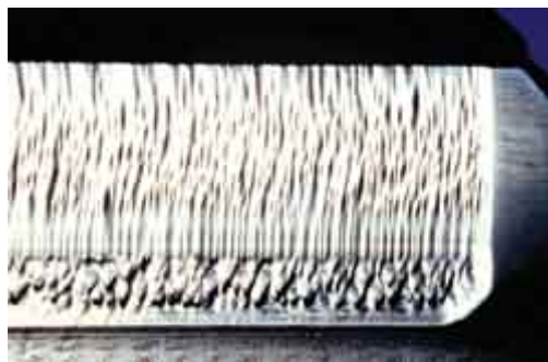
Figure 1. Gear tooth with abrasive wear typical of damage caused by hard particles in the lubricant. (Courtesy of Geartech)
